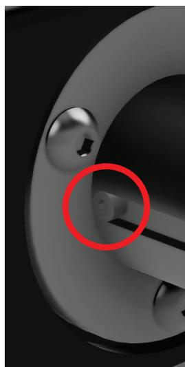
4. Tighten the yoke fixing screw on the bottom of the yoke clamp with the small allen key making sure it is tightened enough to stop any movement. If this is not secure it there will be movement during use which may lead to damage to the connectors or injury to the user.
